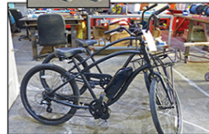
Two black bicycles — the traditional bicycle (rear) is modified to be an e-bike (front).
